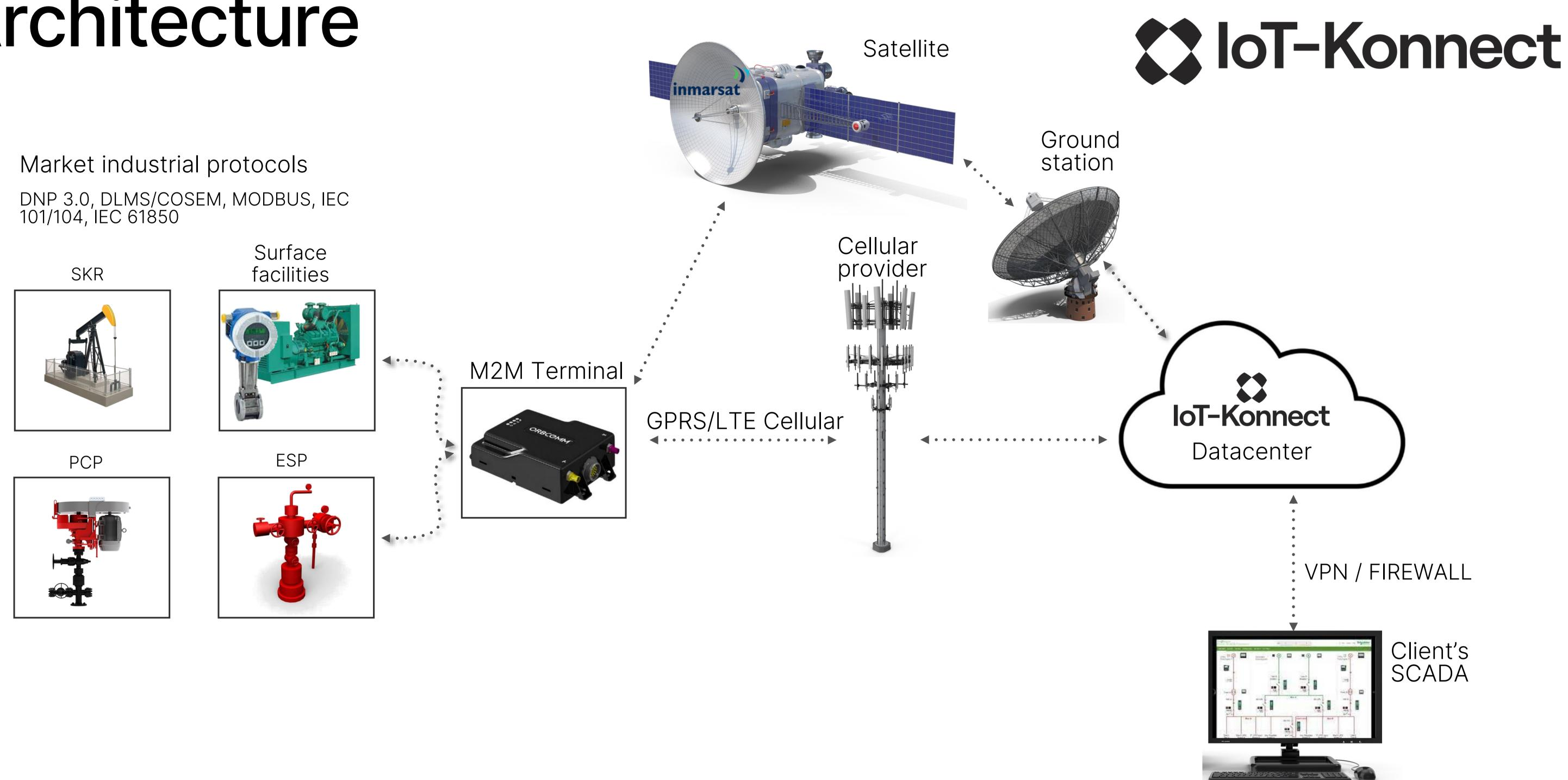
Our M2M terminal installed in the field is fully programmable and is in charge of communicating the slave device with your SCADA or DSS software. The signals are sent through a variety of communications options up to our middleware and then to your SCADA or DSS software, using encrypted and secure channels.
